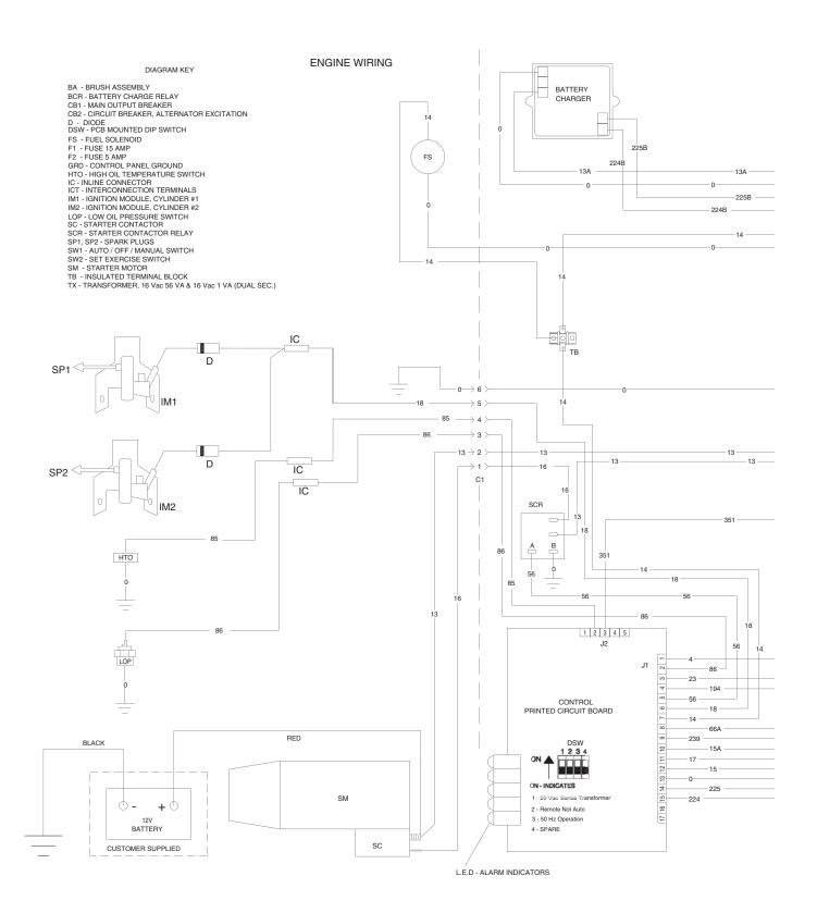
Air-cooled 8.5 kW Generator Wiring Diagram - 8.5 kW - Drawing No. 0D8500-B
